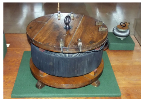
Prototyptransformator på Széchenyi István Memorial Exhibition, Nagycenk, Ungern.
